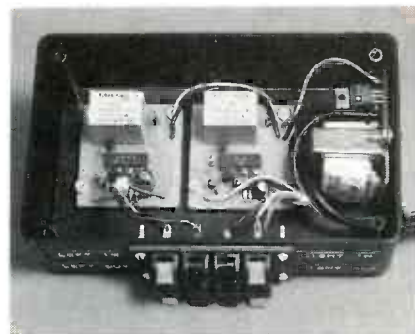
FIG. 7—HERE'S THE AUTHOR'S PROTOTYPE. It contains a protector circuit for both the left and right channels and one power supply. The entire unit is only about 4 inches wide by 6 inches long.
